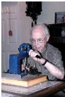
*Don removing a worn bearing. Note cuckoo quail clock on wall.*
